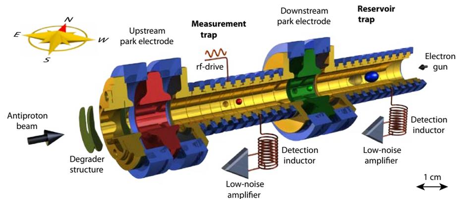
Schematic of a magnetic Penning trap at the Antiproton Decelerator in CERN (European Organization for Nuclear Research).
