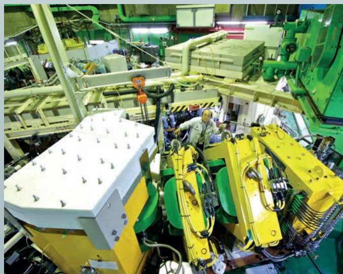
Kosuke Morita's group at the RIKEN Nishina Center for Accelerator-Based Science discovered element 113 using the gas-filled recoil ion separator (GARIS).
