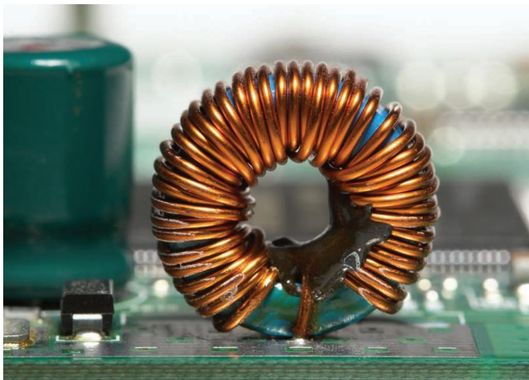
A conventional inductor mounted on a printed circuit board. Inductors have resisted miniaturization until now, but the demonstration of a quantum source of inductance by RIKEN researchers promises to result in much smaller inductors.
