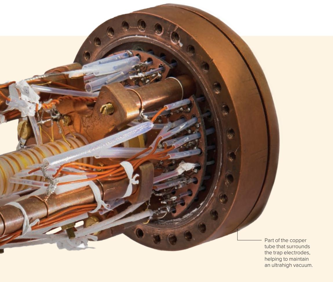
Part of the copper tube that surrounds the trap electrodes, helping to maintain an ultrahigh vacuum.
