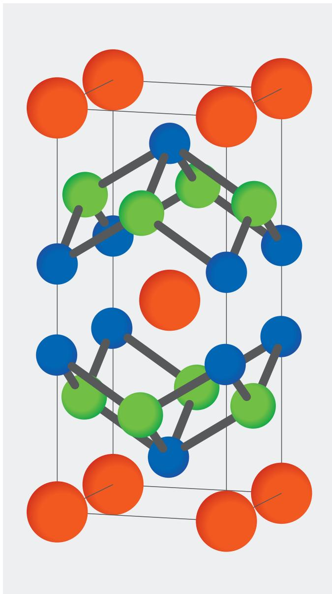
The crystal structure of gadolinium ruthenium silicide, which can host a square lattice of swirling magnetic skyrmions (orange = gadolinium; green = ruthenium; blue = silicon).
