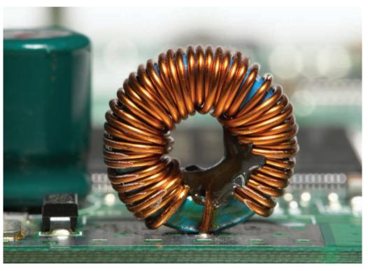
A conventional inductor mounted on a printed circuit board. Inductors have resisted miniaturization until now, but the demonstration of a quantum source of inductance by RIKEN researchers promises to result in much smaller inductors.
