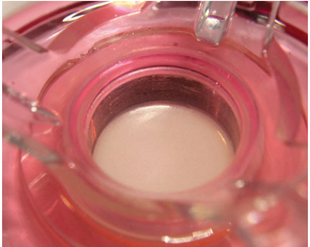
A photograph of an artificial skin developed by RIKEN researchers that reproduces the tension balance of natural skin.
