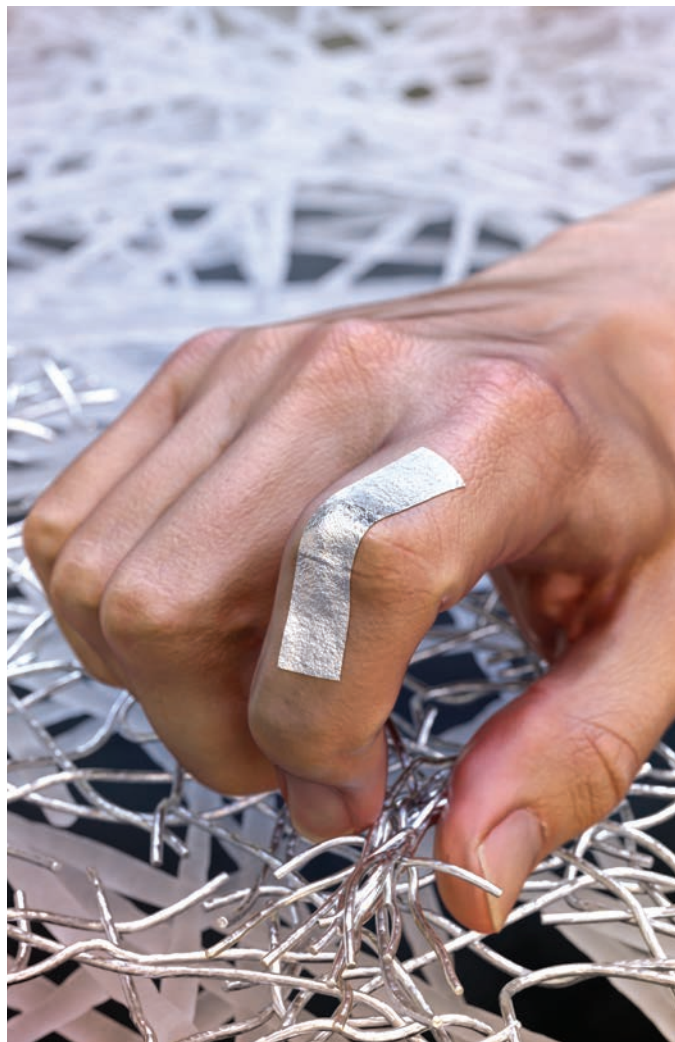
A photo of the film attached to a person’s finger. It can be used as a wearable sensor to monitor heart rate and other movement.
